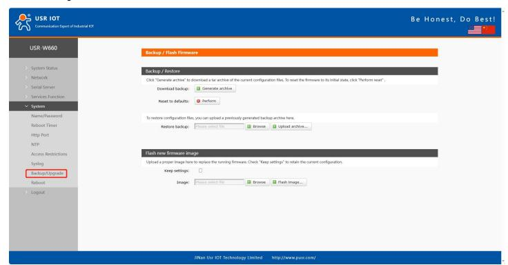
Figure 9. Parameters backup/firmware upgrade
