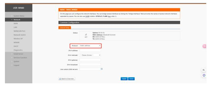
Figure 12. Static IP settings
