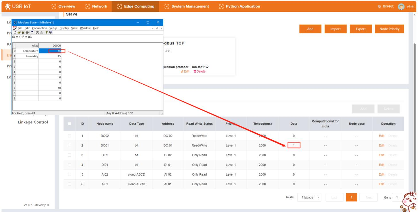
In Normal temperature, if the value of temperature is lower than 45, then turn off DO1.
