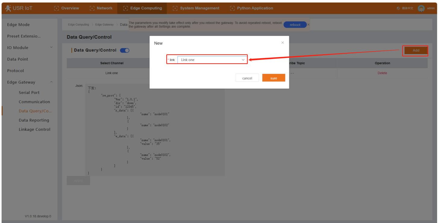
In section 5.4, the added data points have data already, now we can collect the data to the server. Set the Network Assistant as TCP server, the local port is 8234, USR-M300 work as TCP client to connect the TCP server. Then send json command to collect the temperature and Humidity data, to control the level data at the same time. User can copy the json command sample and change the query and control command based on the sample.
