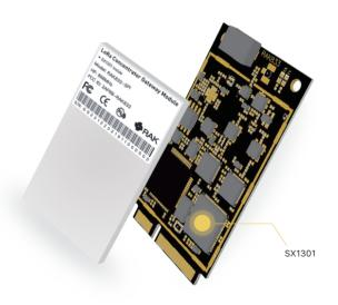
A SPI interface is provided on the PCIe\_SCK, PCIe\_MISO, PCIe\_MOSI, PCIe\_CSN, PCIe\_RST(Reset) pins of the system connector. The SPI interface gives access to the configuration register of SX1301 via a synchronous full-duplex protocol. Only the slave side is implemented.
