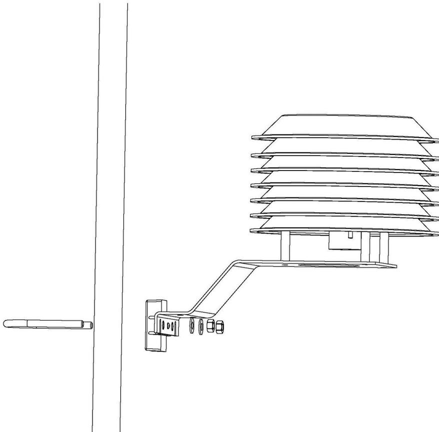
(1) In the position to be installed, loosen the U-shaped screw at the bottom of the R727 device and the mating washer nut, and fix the U-shaped screw through the appropriate size cylinder on the fixed post piece of R727. Fit the shim nut and lock nut in order till R727 device body is not stable shaken.
