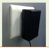
4. The device is compatible with LoRaWAN open protocol class C which enables it to transmit infrared command upon receipt of the downlink command. The device also supports remote controller functions.
