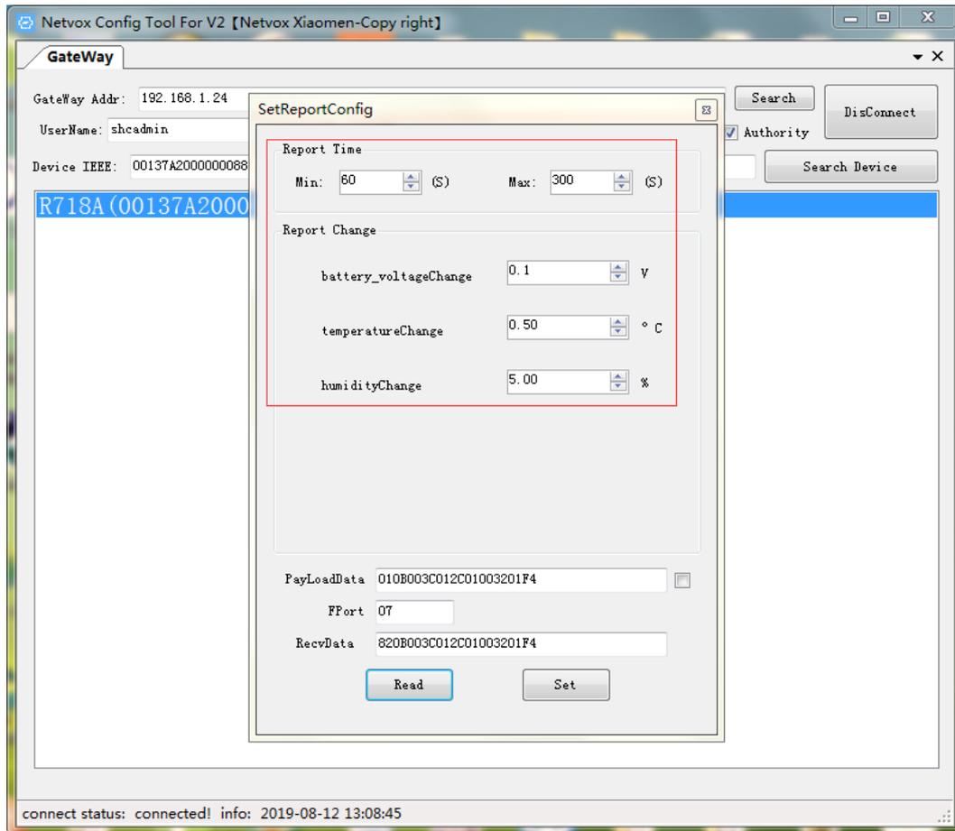
4. If you need to send other supported commands in LoRaWAN, users can tick the PayloadData option, fill in the PayloadData data content, and then click " Set " to send the configuration, as shown in the screen shot below:
