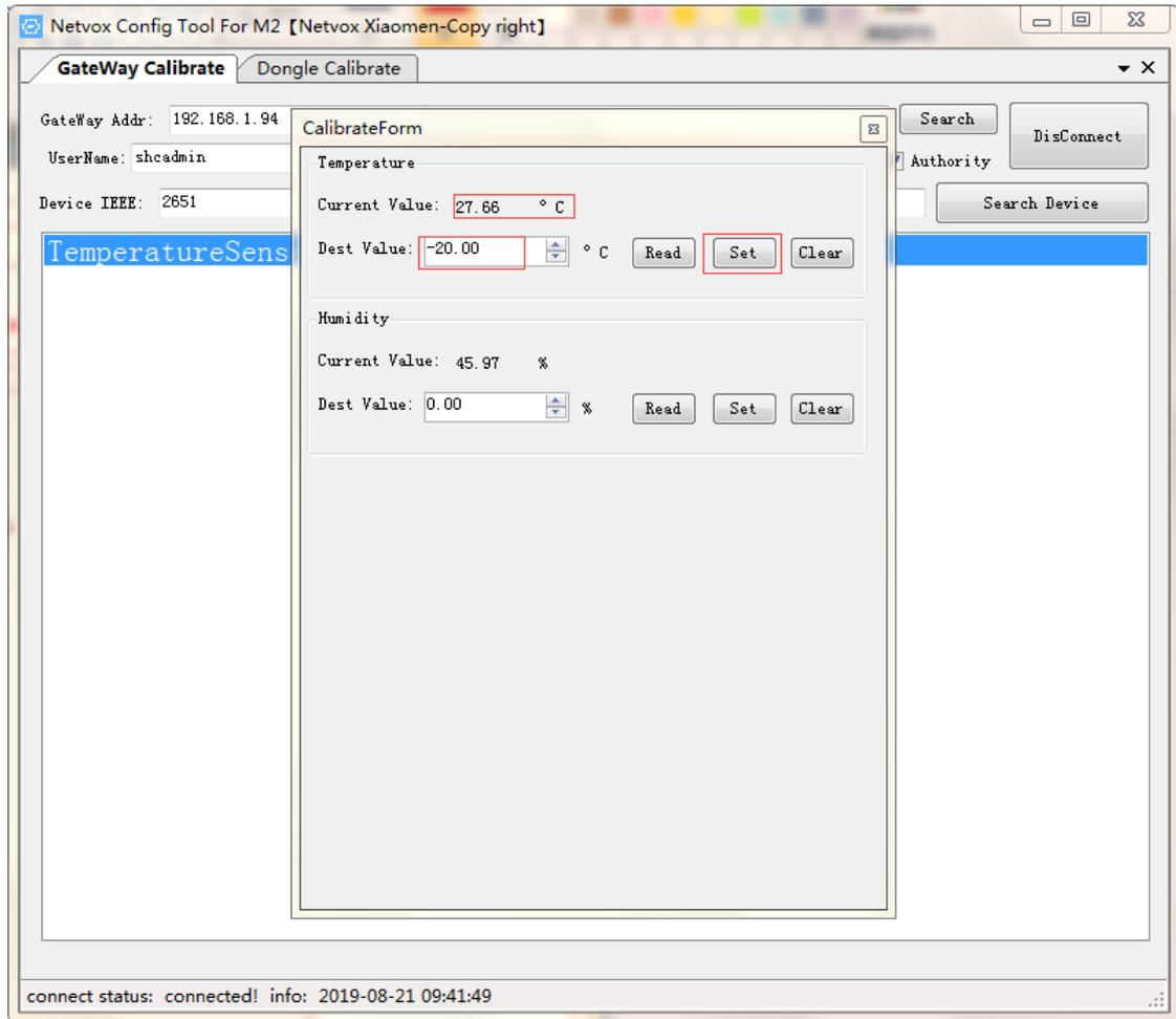
After the calibration is successful, Dest Value will display 0. You can click the “ Read ” button, press the button to activate the device, and read the calibrated Dest Value. At this time, the Current Value returned by the device should be close to the standard source device detection value. The device temperature value is successfully calibrated as shown below:
