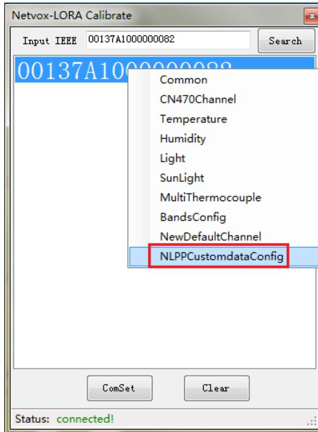
After entering the Customdata modification interface, click the “Read” button to read the current programming value of the device, as shown in the Fig. below:
