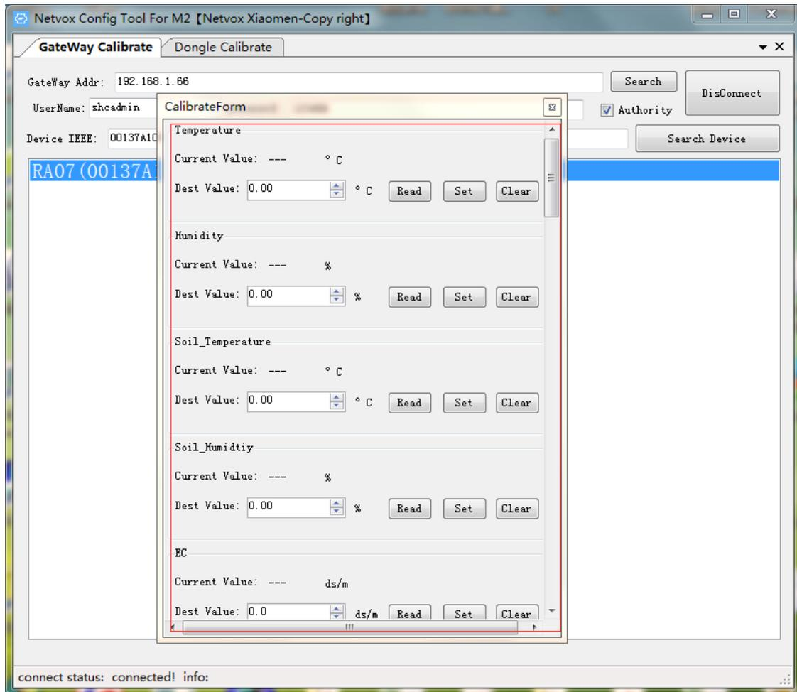
3. Users can press the device button once to wait for the current attribute value of the device to report back. After it is successful, it will be displayed on each corresponding attribute position on the tool, as shown in the following figure:
