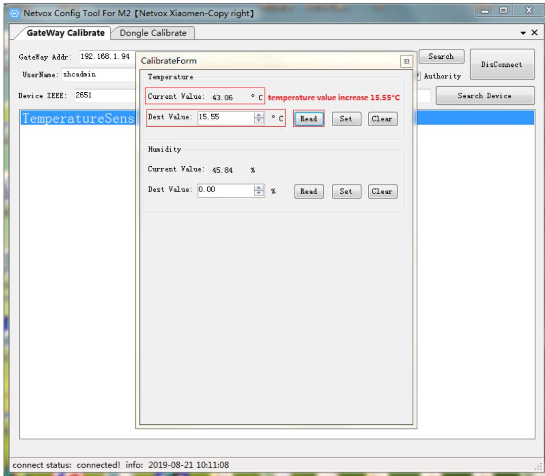
6. If the difference between the standard source device detection value and the current device detection value is negative, the input value in the Dest Value input box should be filled with a negative value. As shown in the figure below, the temperature value is reduced by 20° C, Dest Value=-20° C . Then click the “ Set ” button, and when the prompt box pops up **send success ! please active the device...** , press the button to activate the device.
