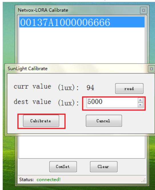
3.2.4 After the calibration is completed, click the "read" button again to get the return value after the calibration of the device. As the following Fig. in below, the sunshine value returned after calibration is: 4953 lux, which has been modified to the
