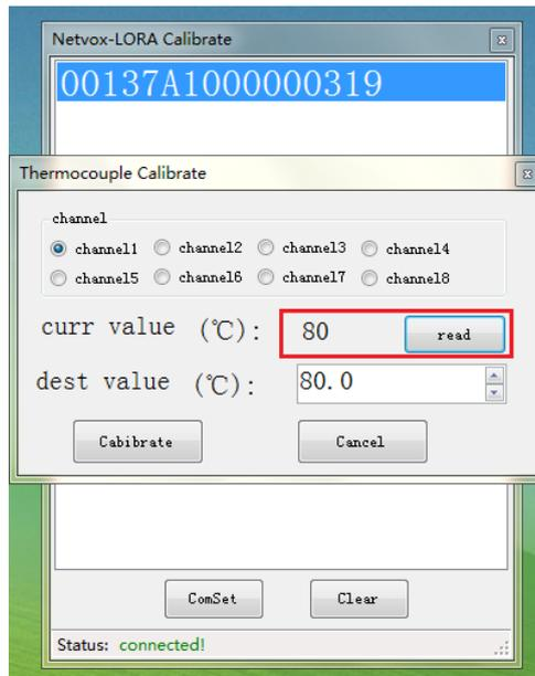
The calibration of other channels is the same. The calibration operation of other attributes is the same as the attribute calibration operation of the example. It is not repeated. After the device attribute value is successfully calibrated, power on and power off to enter normal working mode.
