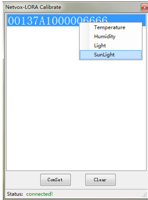
3.2.2 Enter the sunshine property calibration interface, click the “read” button to get the sunlight value returned by the current sampling device, as shown in the Fig. below:
