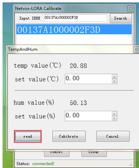
3.1.3 When the user thinks that the temperature and humidity values are incorrect and need to be calibrated, enter the standard temperature value in the temperature calibration input box, and enter the standard humidity value in the humidity calibration input box. For example, enter the temperature value: 30.50, enter 60.80 in humidity value and click “Calibrate” button to write the calibration values as shown below:
