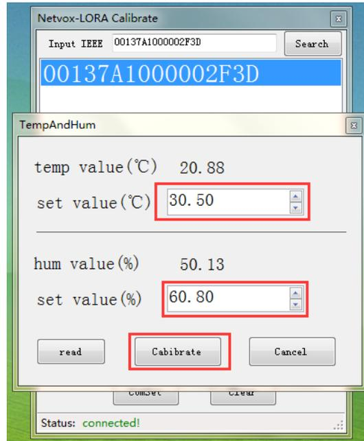
3.1.4 During the calibration process, the button will become gray and unavailable. After the calibration is completed, the button color will be restored. Click the “read” button to read the temperature and humidity value after the calibration of the device.
