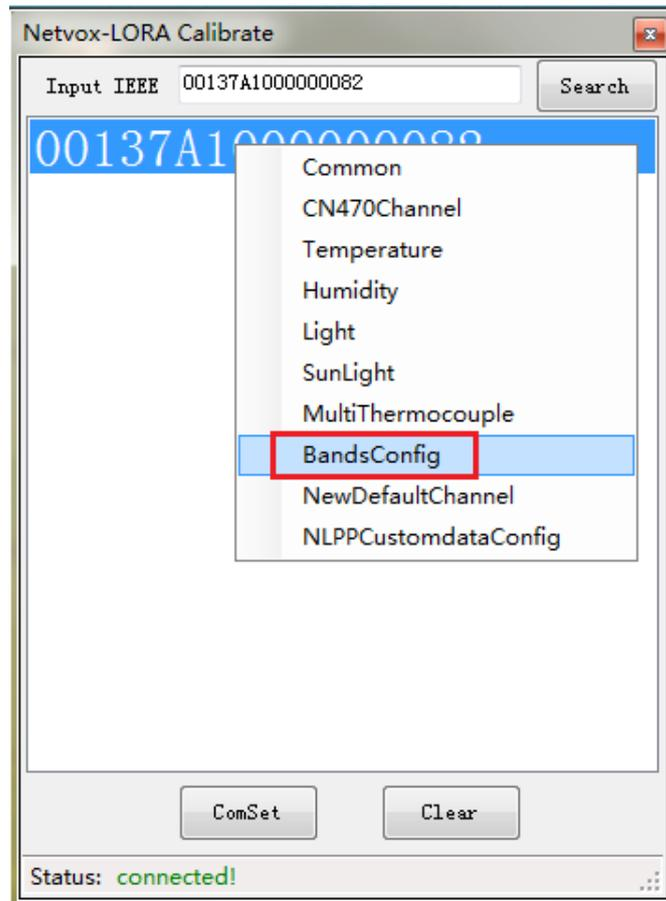
After entering the Band modification interface, click the “Read” button to read the current Bands information of the return device. The default device shipment is usually band1~band8, as shown in the Fig. below:
