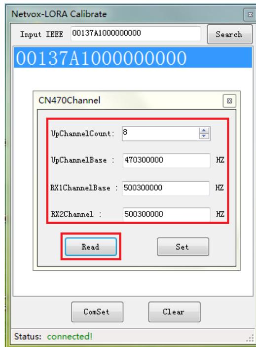
Input device uplink frequency point UpChannelCount, the default value is generally 8 frequency points; input the uplink starting frequency point UpChannelBase; note that the unit here is HZ; input the downlink starting frequency point RX1ChannelBase; input the downlink RX2Channel frequency point, and then click "Set" button to enter the set value. After the setting is successful, there will be an “operate success”
