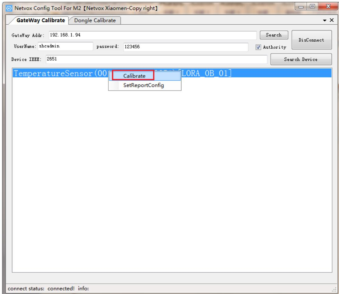
2. Enter the calibration interface, taking the R718A device temperature value calibration as an example. The current value of the device property is not retrieved, and " --- " is displayed, as shown in the following figure:
