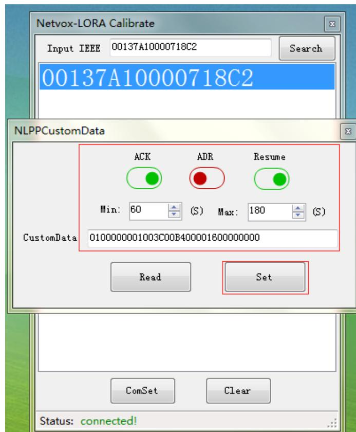
After selecting the desired setting item, click the “Set” button to write the device. After the setting is successful, there will be “operate success” window prompt, or click the “Read” button to read the information returned after setting, as shown below:
