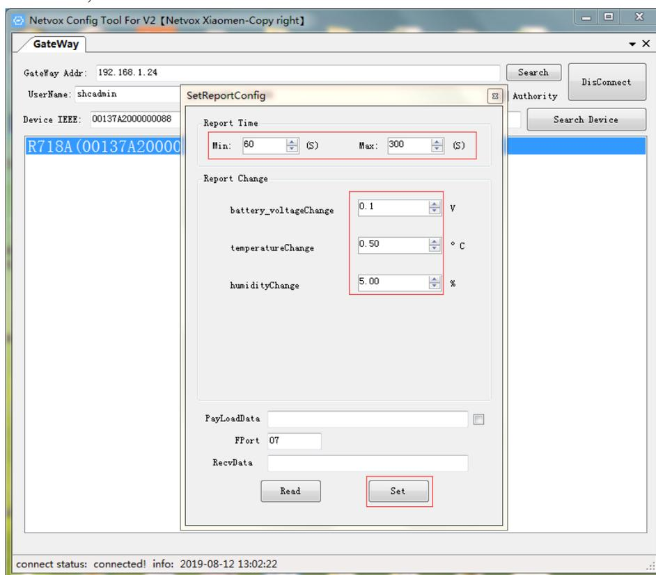
Fill in the parameters to be modified, and finally click the “ Set ” button to issue the configuration command. In the pop-up **send success ! please active the device...** prompt box, the command is sent successfully. Users need to press the R718A device button once to activate the device to receive the command. After the device is configured successfully, all the input boxes on the interface will display 0, as shown in the following screen shot:
