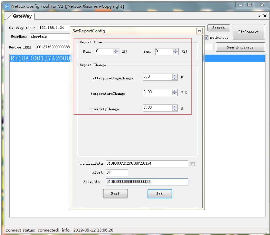
At this point, click the “ Read ” button, press the device button once to activate the device. After reading successfully, return the configured value as shown in the screen shot below:
