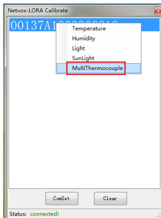
3.3.2 After entering the thermocouple calibration interface, firstly select the way to calibrate the thermocouple. Selects “ channel1 ” for the first thermocouple temperature calibration. Select “ channel2 ” for the second thermocouple temperature calibration , and so on.
