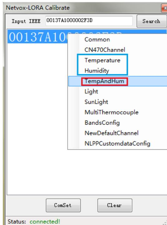
3.1.2 Enter the temperature and humidity value calibration interface, click the “read” button to read the temperature and humidity values currently collected by the device, as shown below:
