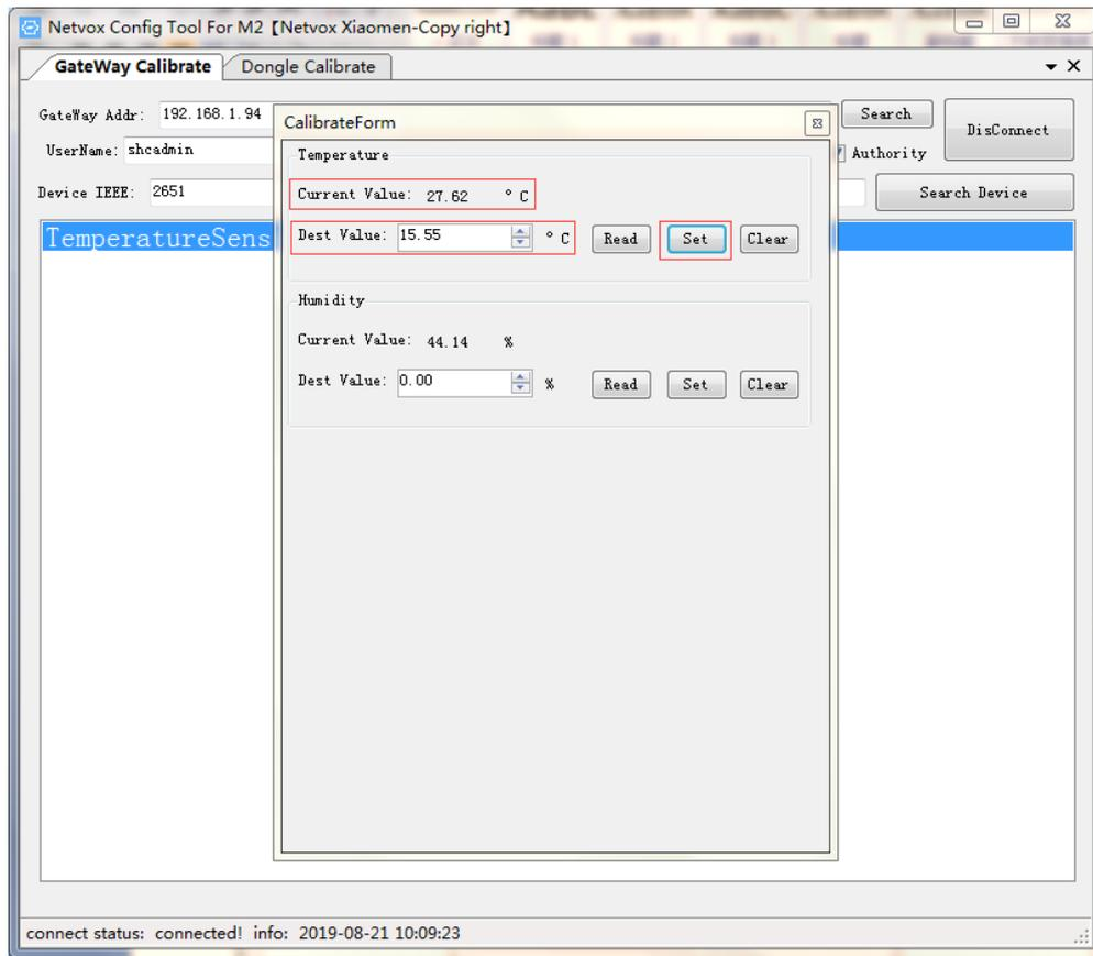
After the calibration is successful, Dest Value will display 0. You can click the “ Read ” button, press the button to activate the device, and read the calibrated Dest Value. At this moment, the Current Value returned by the device should be close to the standard source device detection value. The device temperature value is successfully calibrated as shown below:
