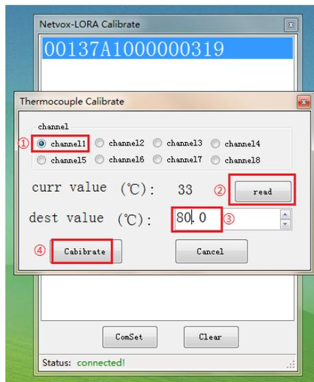
3.3.3 After temperature value calibration is successful, click the “read” button again to re-read the return value after calibration. As shown in the figure below, the read temperature value of the first channel of the thermocouple has been calibrated to the standard source temperature value 80 ° C and so on.
