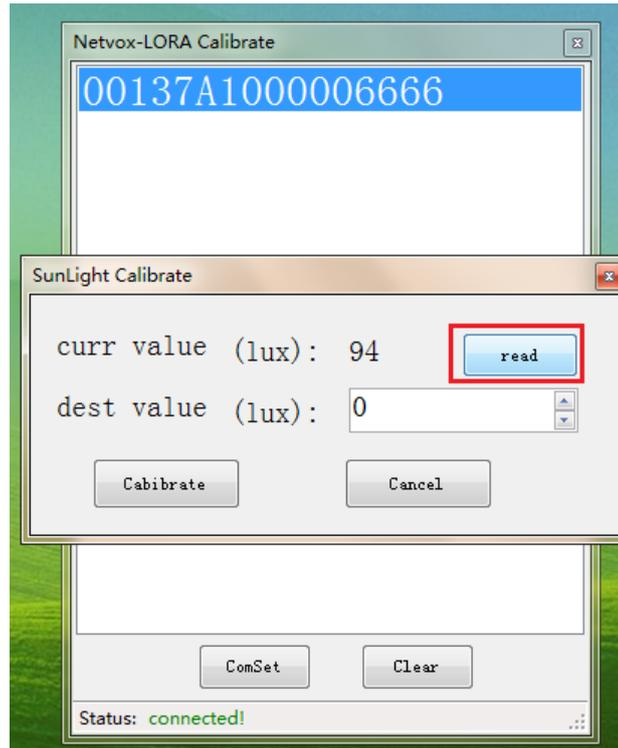
3.2.3 When the current value returned by the device is not accurate enough compared with the value measured by the standard source, the calibration can be made. For example, if the standard source value indicates that the current sunshine value should be 5000 lux, the dest value input box should be filled in 5000. Then click on the "Calibrate" button to write the calibration value, as shown in the Fig. below:
