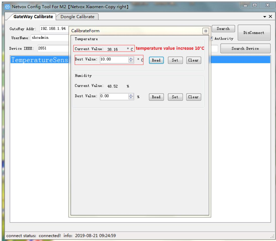
5. If the current value of the device is found to be much worse than the standard source detection value after calibration, users can click the “ Clear ” button. Press the device button once to activate the device, and clear the calibration correction value. After success, the Dest Value value will display 0 . Fill in the new difference in the Dest Value input box, as shown below, fill in the value of Dest Value at 15.55 ° C , and then click the “Set” button. When the prompt box pops up
