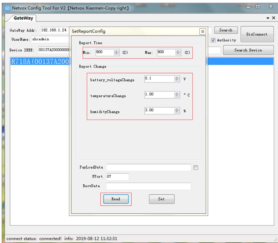
R718A factory default Min=900s, Max=900s, battery\_voltageChange=0.1v , temperatureChange=1.00 ° C , humidityChange=3.00%
