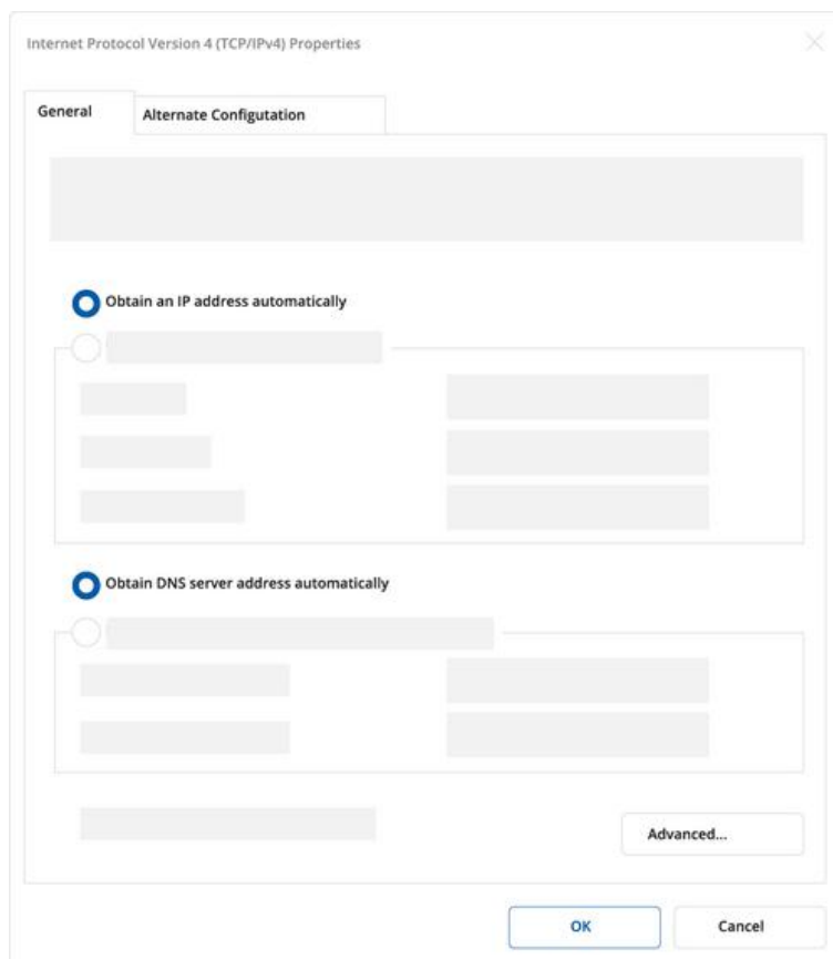
Fig. 13 Configure the IP address of PC
