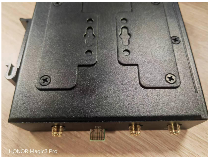
Fig. 9 Install the sim card
