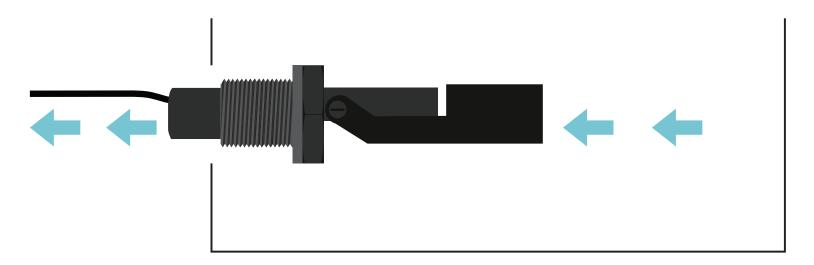
Now that the float switch is in place, re-attach and fully tighten the blukhead.
