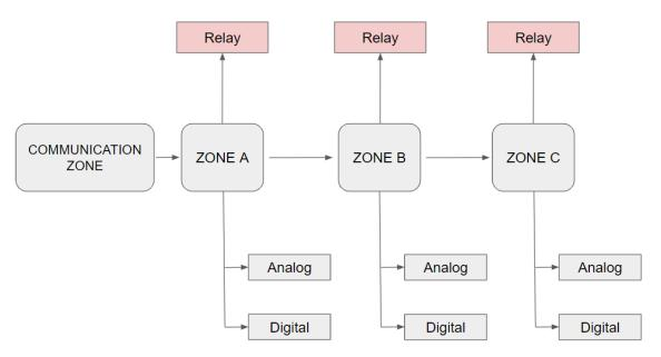
This is the possible zones scheme, whether the zone is Analog/Digital or Relay depends on your device, you can consult it on the <u>Zones Table</u>. The distribution of the different features that provide the Raspberry PLC Family are described below.
