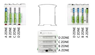
• The inputs in the zone A/B/C are named IX.X, being X any number suitable in the Shield. Outputs are named as QX.X.
