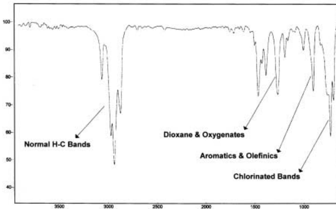
A sample of a highly contaminated waste lube oil showing halogenated solvents (chloroform, chloroethyleness), aromatics (benzene, toulene, xylene), dioxanes, and ethers. Data comes from a three-minute scan.
