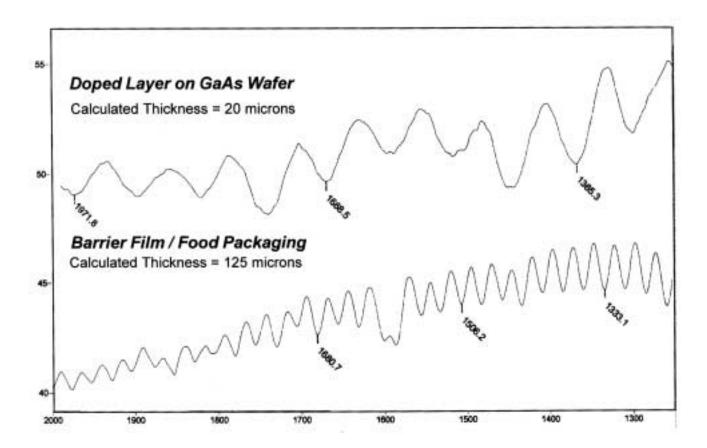
The gallium arsenide wafer was run by transmission using a modified film holder and a "map" was made to verify the uniformity of the doping throughout the wafer. The barrier bag film was scanned using the magnetic film holder.
