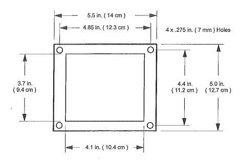
**Blower Motor Exhaust Flange and Mounting Holes**
