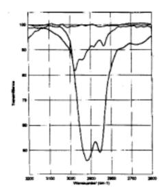
Infra-red scan showing typical hydrocarbon stretch in the 2800 - 3050cm<sup>-1</sup> region.
