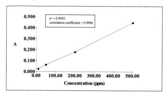
**Analysis:** Total Petroleum Hydrocarbons by Infrared Spectroscopy (EPA 418.1)
