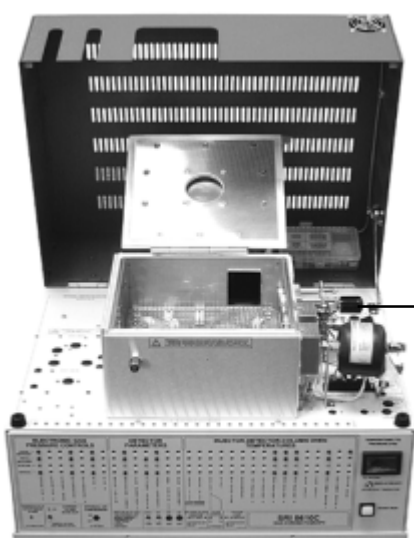
PID in series with a DELCD and an FID on a 910 chassis
