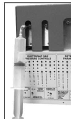
Injection by syringe of gas sample into valve
