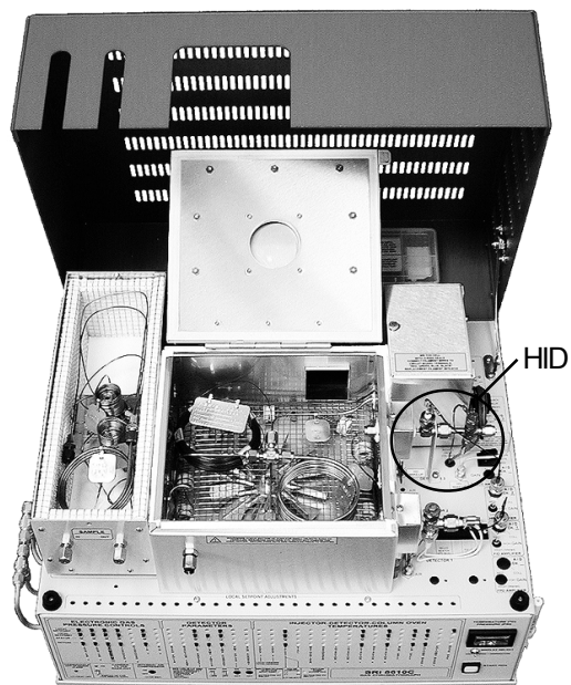
HID detector between TCD and FID detectors
