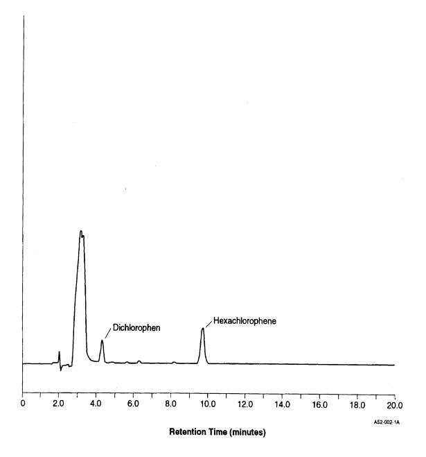
Figure 1. HPLC-UV Chromatogram of 10 ng Each of Hexachlorophene and Dichlorophen (Column 1)
