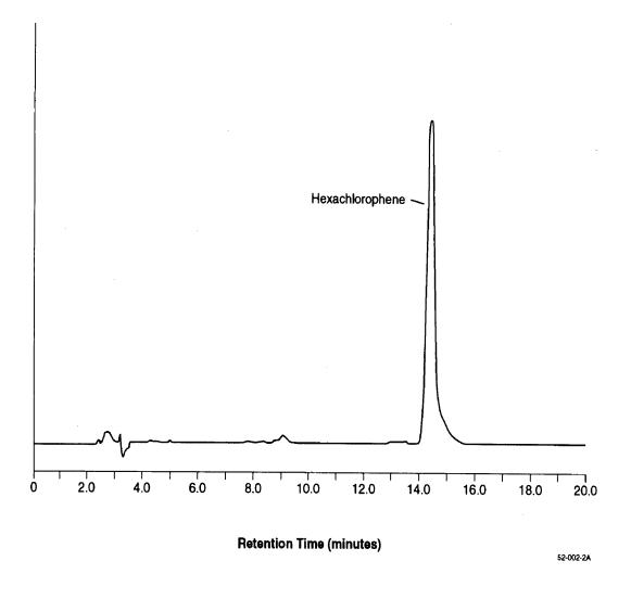
Figure 2. HPLC-UV Chromatogram of 250 ng Each of Hexachlorophene (Column 2)
