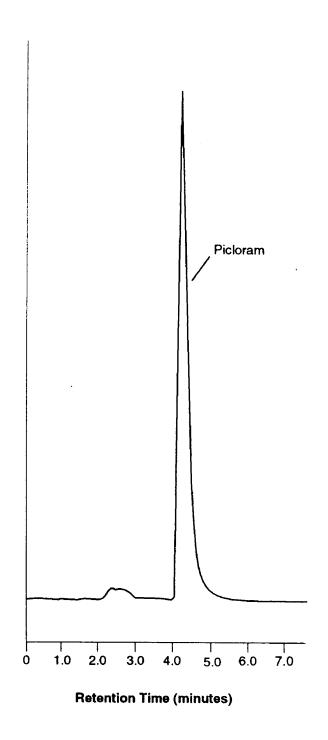
Figure 2. HPLC of Picloram in Wastewater Extract
