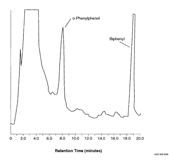
Figure 1. Liquid Chromatogram of Wastewater Extract Fortified With o-Phenylphenol and Biphenyl (Column 1)
