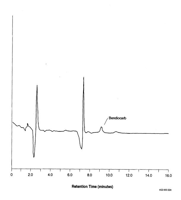
Figure 1. HPLC-UV Chromatogram of 10 ng of Bendiocarb (Column 1)
