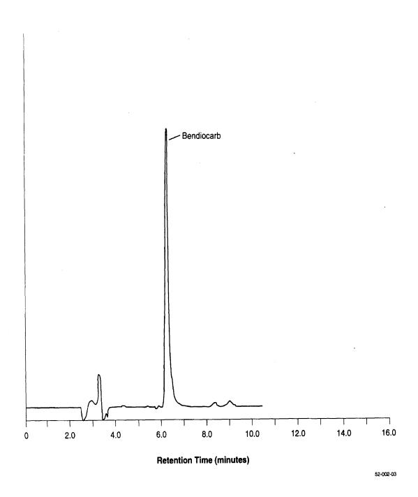
Figure 2. HPLC-UV Chromatogram of 600 ng of Bendiocarb (Column 2)
