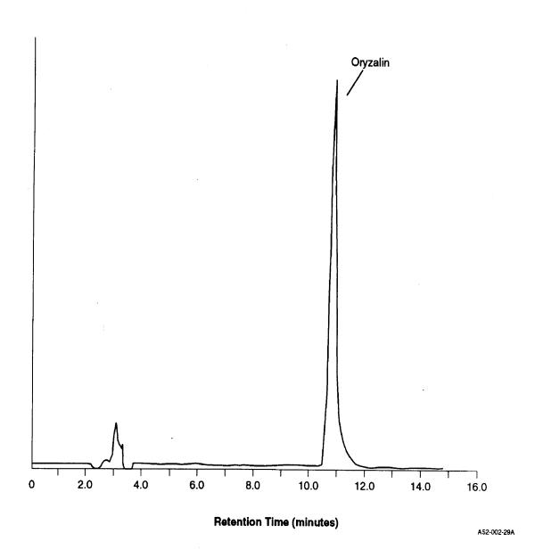
Figure 2. HPLC-UV Chromatogram of 250 ng of Oryzalin (Column 2)
