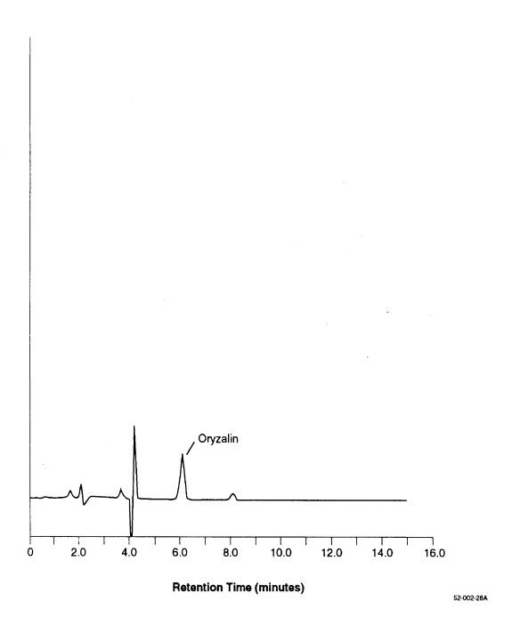
Figure 1. HPLC-UV Chromatogram of 10 ng of Oryzalin (Column1)
