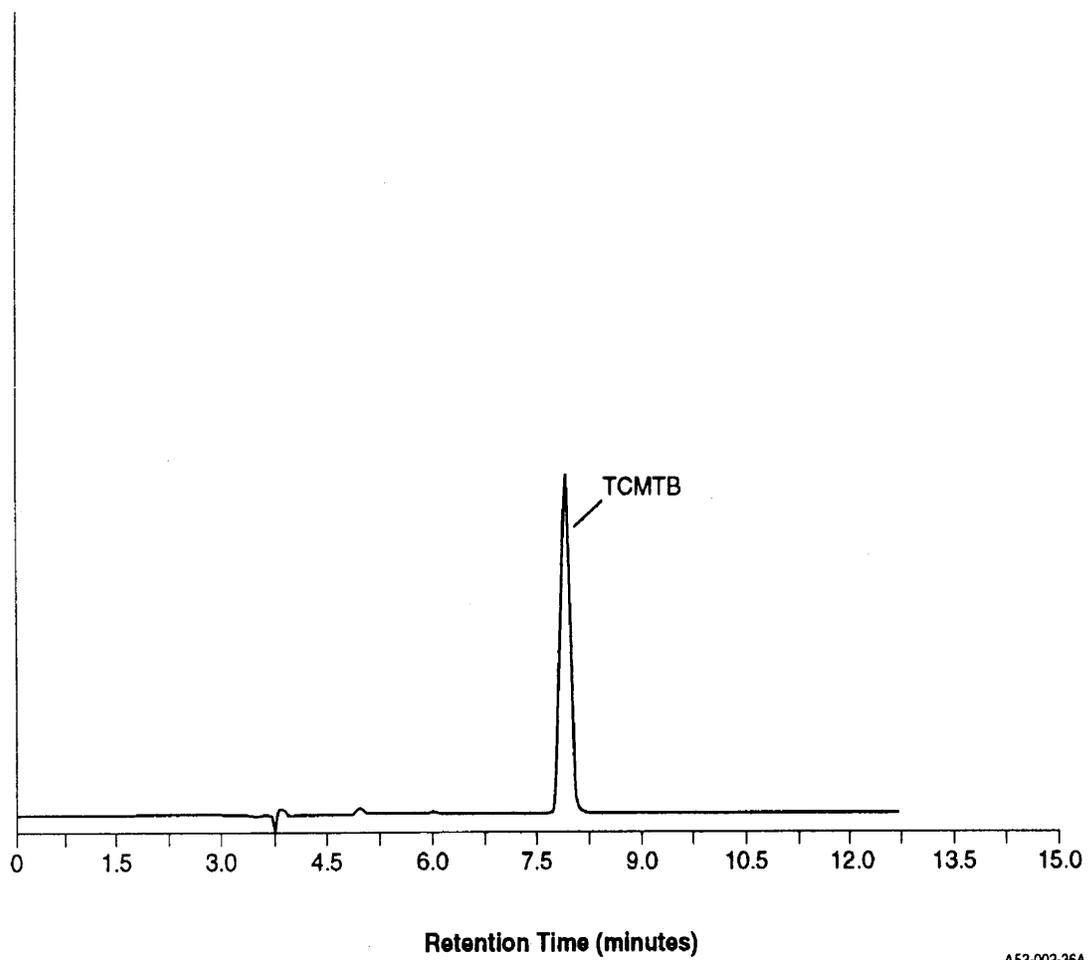
Figure 3. HPLC-UV Chromatogram of 100 ng of TCMTB (Column 2)
