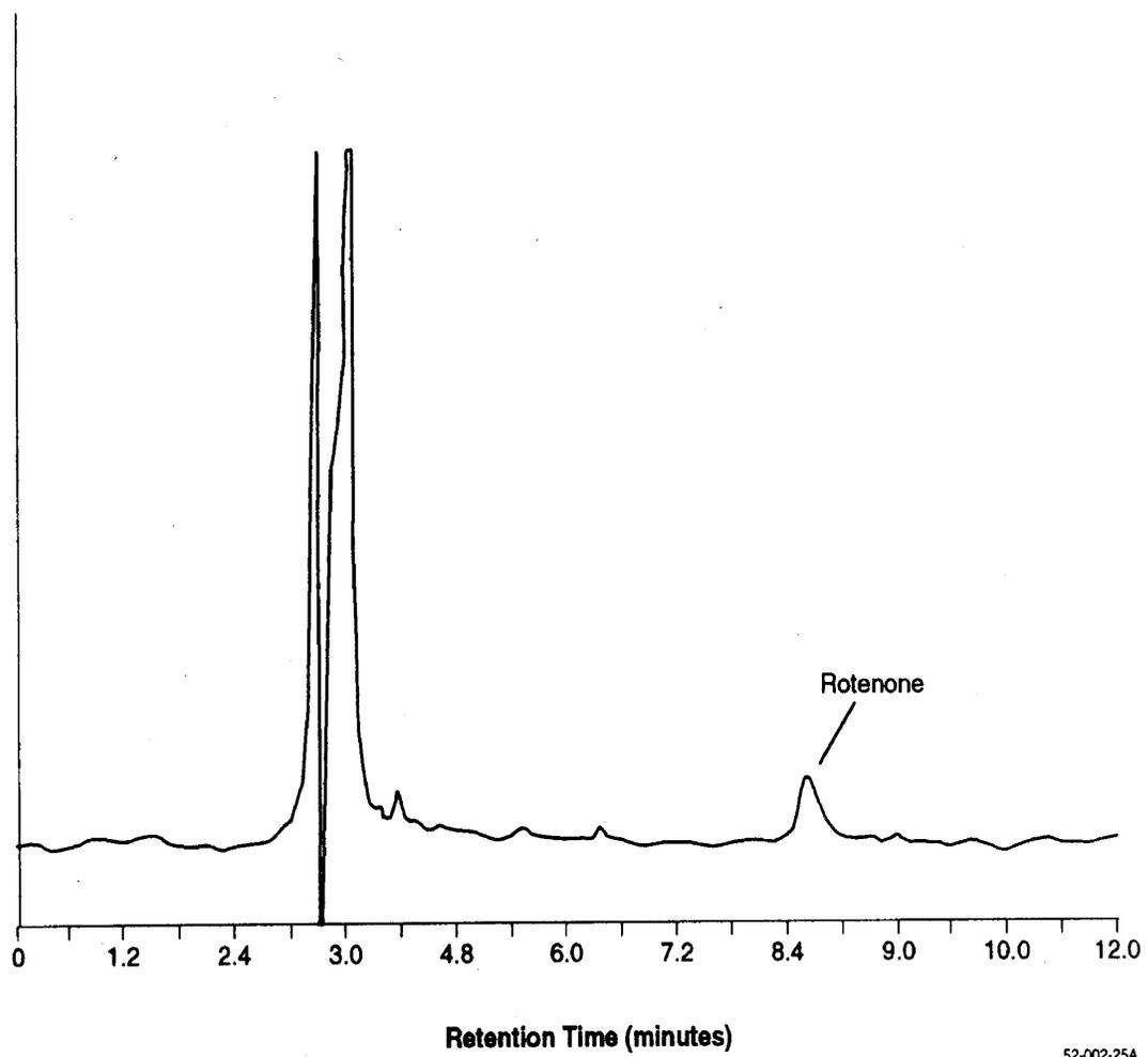
Figure 1. HPLC-UV Chromatogram of Standard Solution Representing 5 µg/L of Rotenone in Water (Column 1)
