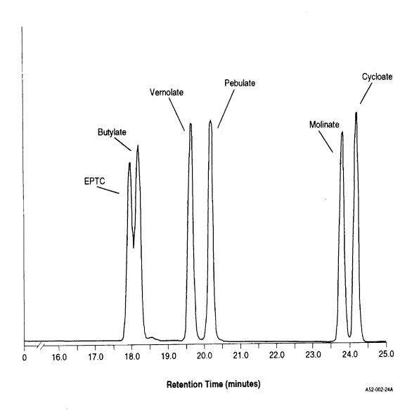
Figure 2. GC-AFD Chromatogram of 200 ng of Each Thiocarbamate (Column 2)
