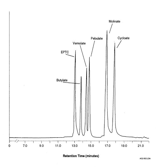
Figure 1. GC-AFD Chromatogram of 200 ng of Each Thiocarbamate (Column 1)
