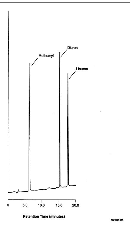
Figure 1. Liquid Chromatogram of Diuron, Linuron and Methomyl on Column 1 (for conditions, see Table 1)
