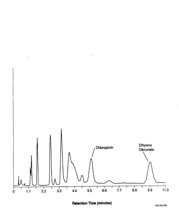
Figure 1. GC-ECD Chromatogram of 200 ng Chloropicrin and Ethylene Dibromide in Cyclohexane (Column 1)
