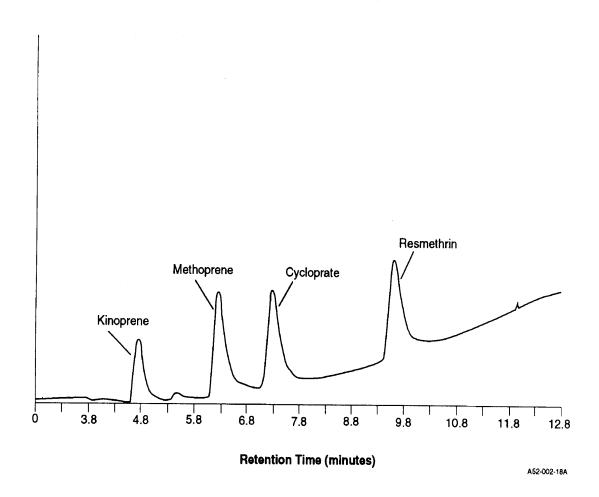
Figure 2. GC-FID Chromatogram of 200 ng Each of C, H, and O Compounds (Column 2)
