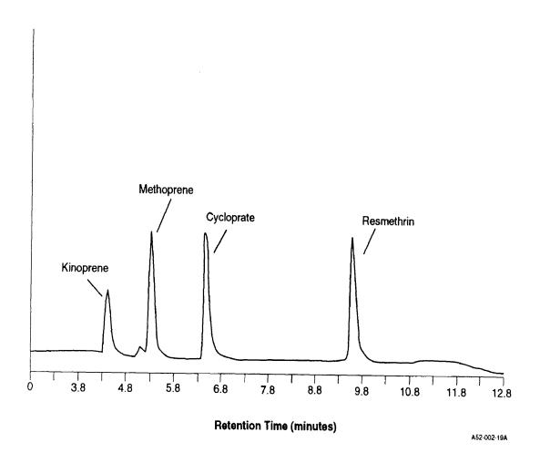
Figure 1. GC-FID Chromatogram of 200 ng Each of C, H, and O Compounds (Column 1)
