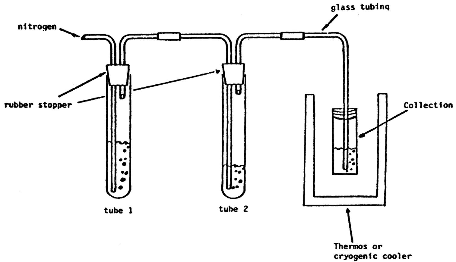
FIGURE 2. DIAZOMETHANE SOLUTION GENERATOR
