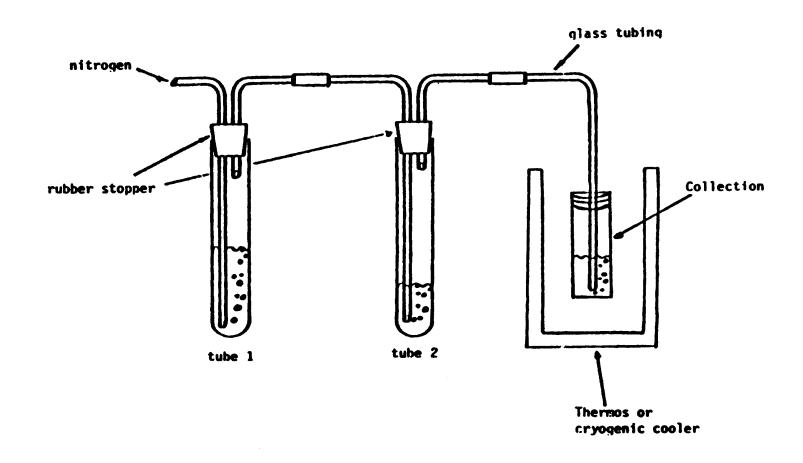
FIGURE 2. DIAZOMETHANE SOLUTION GENERATOR
