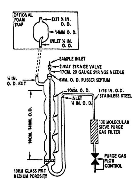
FIGURE 1. PURGING DEVICE
