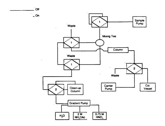
Figure 2. System Diagram without Sample Loop.
