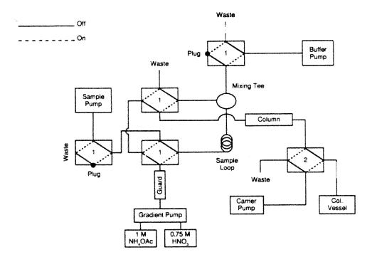
Figure 1. Sample Loop Configuration.
