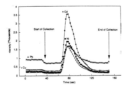
Figure 3. Peak Collection Window from ICP-AES.
