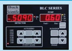
6 Different wavelength filters to choose from for your single pump workhorse! 254nm~280nm~365nm~420nm~505nm ~540nm Filter and source kits available for wavelength changes in the field.
