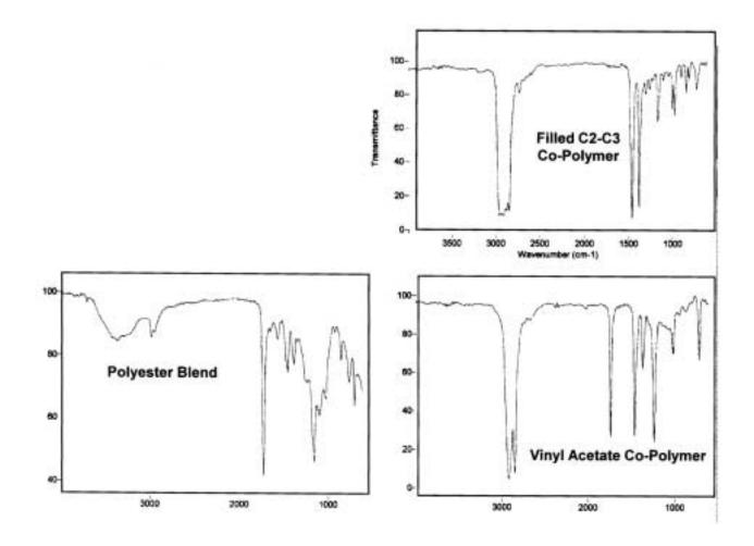
Three typical polymer materials scanned by reflectance ATR using the Model 59 Vertical ATR with a KRS-5 crystal. Using the GRAMS/IR software with advanced spectral manipulations, data can be formatted into a wide variety of presentations.
