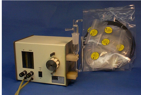
Model-420 unit with Glassware mounted and bag of Installation components
