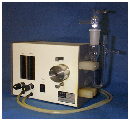
Attach U-Tube and Phase Separator Glassware CAREFULLY! It is fragile and can be easily damaged if bumped!
