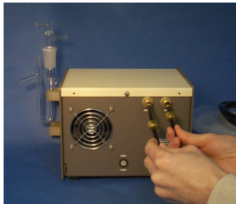
Connect AIR and ARGON Lines to back of unit using included 1/4\" Swagelok Compression Fittings on Nylon tubing
