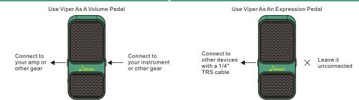
When using your Viper as an expression pedal, connect the OUTPUT jack to your device's expression pedal INPUT jack with a TRS (Tip-Ring-Sleeve) cable, and LEAVE THE INPUT JACK UNCONNECTED. We recommend you to use a cable with TRS plugs ON BOTH ENDS (at least the plug connected to the unit should be a TRS end).
