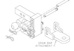
**STEP 1:** PUT TOW & STOW RECEIVER HITCH INTO "STOW" POSITION. **STEP 2:** POSITION DRAW BAR ATTACHMENT AS SHOWN AND ALIGN IT WITH TWO HOLES IN THE RECEIVER HITCH.
