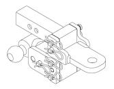
**STEP 3:** ATTACH DRAW BAR TO HITCH WITH BOTH PINS PROVIDED AND SECURE THE PINS WITH THE INCLUDED HAIR PINS.
