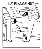
FIGURE B5: View looking up at the inside of passenger side frame.
