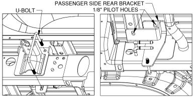
FIGURE A6: View looking up at the outside of passenger side frame.
