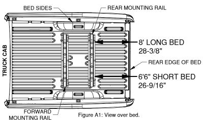
The fuel tank of the truck may be directly below the area of the bed which needs to be drilled. Always carefully examine the area under the truck where drilling will occur before drilling. Make certain that the tank, or other equipment, is not damaged during drilling. Damage to the tank may result in property damage, serious injury or death.
