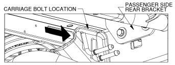
FIGURE C7: View looking at passenger side frame and bed crossmemeber Arrow indicates access area
