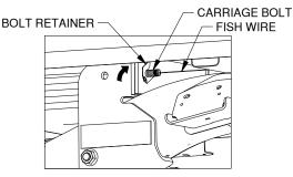
Figure F5: Carriage bolt installation.
