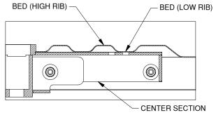
Figure I1: Cutaway view of bed and center section.
