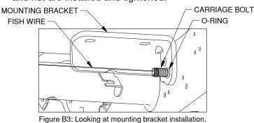
5. Secure hardware. Remove the fish wire from the carriage bolt and secure the bolt with a lock washer and finish nut.
