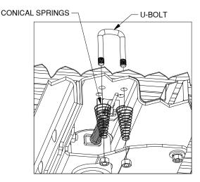
Figure I3: Cutaway view of bed and center section.
