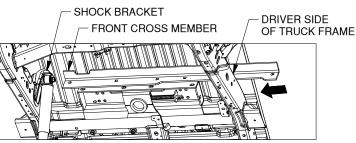
Figure E1: Looking up at center section. (Fuel tank not shown.)
