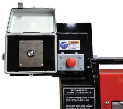
1 BUCKER SPEED CONTROL PANEL & EMERGENCY STOP BUTTON STATIONS 1 & 2
