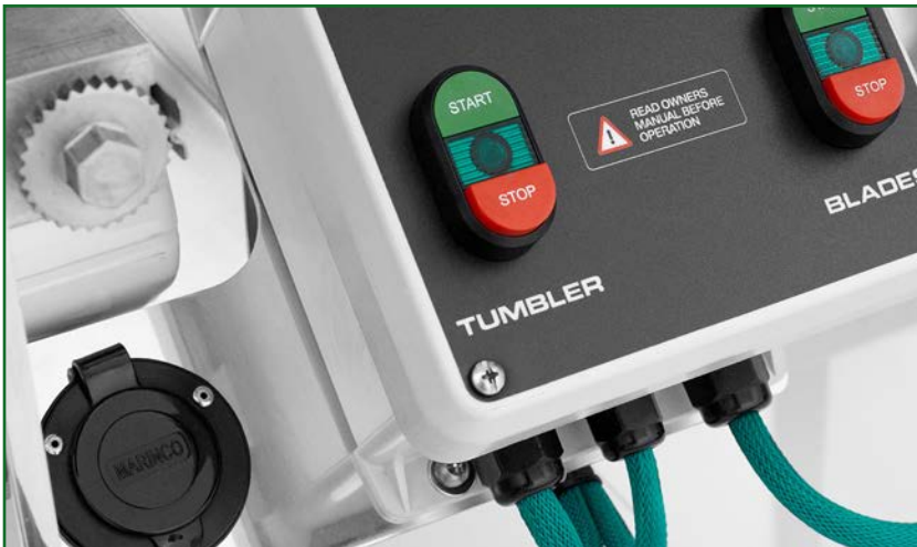
Figure 1.9 Power connection and Switches
