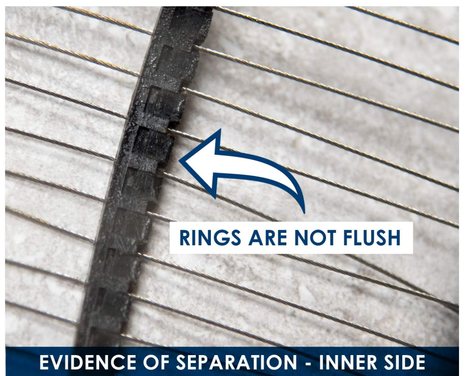
3. INSPECT NYLON RINGS FOR SIGNS OF BREAKDOWN. THE RINGS SHOULD NOT SHOW ANY SIGNS OF SEPARATION ON THE OUTER SIDE OR GAPS BETWEEN RINGS ON THE INNER SIDE.
