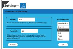
Fixture Models: Choose the correct fixture model for connection. Both wired and wireless connections are suitable for Spectrum-Y.
