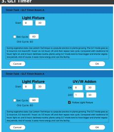
The GLT Timer is a specific mode that works on a 24-hour cycle.
