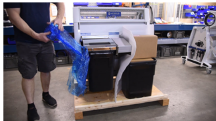
5. Remove blue plastic wrap holding additional components to the body of the machine (Spring Jack Tool, and extra Trim Tote)
