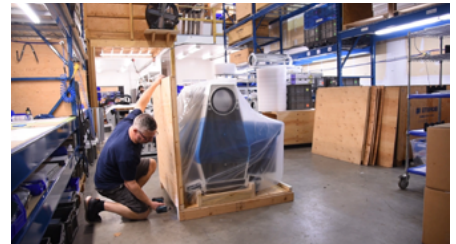
3. Remove 3 remaining side panels
