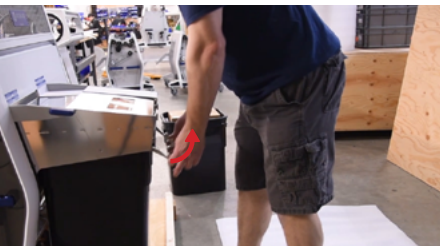
7. Pull up on levers holding the installed trim tote and rotate them downwards
