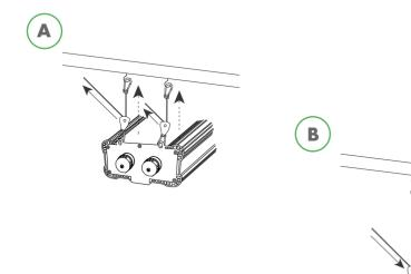
Lift the LED and attach the carabiners to pre-installed hooks from ceiling or mounting beam. The Ratchets should be installed closest to the LED (and not the ceiling).
