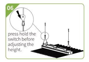
•Adjust the height by pull the cable.
