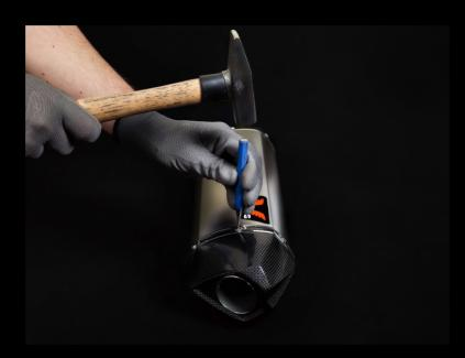
To remove the rivets you must first punch in the middle of the rivets so they become hollow (see the picture above). IMPORTANT: make sure the rivets are hollow (they have a hole in them), otherwise you will encounter problems when drilling out the rivets!
