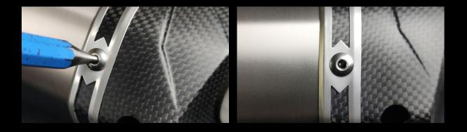
Repeat the punching in process for the other rivets. When that is completed you can continue with the replacement process.
