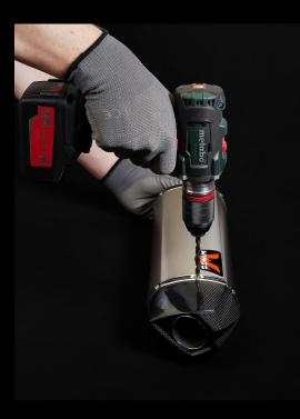
Use a 5 mm drill to drill the rivets out. Remove the carbon end cap and position the new one using a rubber hammer. When in position, put the metal strip back on and rivet everything together with the included rivets.
