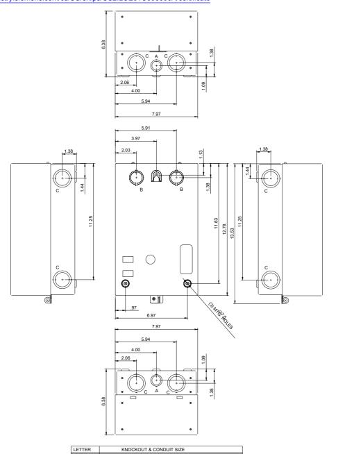
%C22.2 X %C28.6 FOR 12.7 & 19 CONDUIT %C28.6 X %C34.9 FOR 19 & 25.4 CONDUIT %C34.9 X %C43.6 FOR 25 4 & 31.8 CONDUIT
