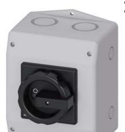
SENTRON, Switch disconnector 3LD, main switch, 6-pole, lu: 25 A, Operating power / at AC-23 A at 400 V: 9.5 kW, molded-plastic encapsulation for metric screw connection, 1 NC, 1 NO, rotary operating mechanism, black
