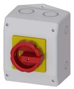
SENTRON, Switch disconnector 3LD, emergency switching-off switch, 6- pole, lu: 25 A, operating power / at AC-23 A 400 V: 9.5 kW, Molded plastic encapsulation for metric cable gland, rotary operating mechanism, red/yellow
