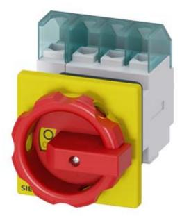
SENTRON, Switch disconnector 3LD, emergency switching-off switch, 4- pole, lu: 25 A, operating power / at AC-23 A 400 V: 9.5 kW, front-mounted, rotary operating mechanism, Red / yellow, central mounting 22.5 mm of the handle
