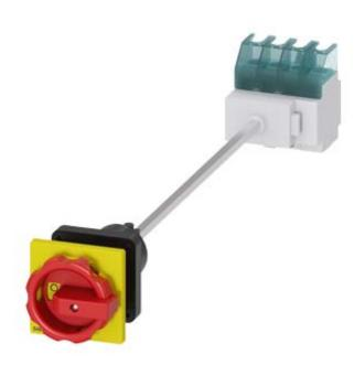
SENTRON, Switch disconnector 3LD, emergency switching-off switch, 4- pole, Iu: 25 A, operating power / at AC-23 A 400 V: 9.5 kW, floor mounting with door coupling, rotary operating mechanism, Red / yellow, central mounting 22.5 mm of the handle
